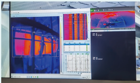
Adding infrared thermal imagers to rotary kilns and material pits
